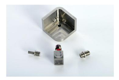
The SA 44 adapter allows you to calibrate the SV 3023M2 accelerometer in all directions.
