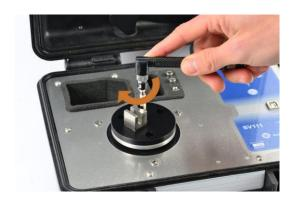
• Dismantle the support system from the case holder, place it on the adapter and tighten the fixing screw.
