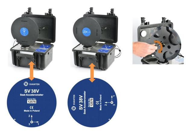
When calibrating axis 3, place the support system with the tested sensor in the horizontal position on the adapter and tighten the fixing screw.
