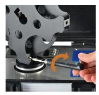
• Unscrew the central screw of the whole-body sensor and mount the sensor on the support system using the <u>10mm short</u> screw.
