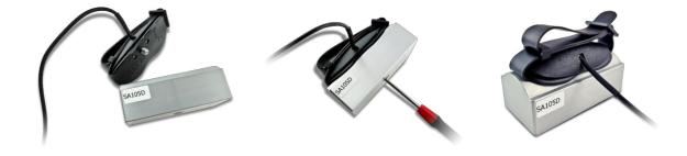
Attach the calibration adapter with the vibration sensor to the calibrator's shaker using the special stud (supplied in the SV 105 kit.
