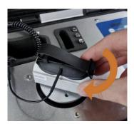
The positioning of the adapter with the sensor for calibration of the X-axis, Y-axis and Z-axis should be as shown in the photos below. For this use the appropriate hole in the adapter for the stud.
