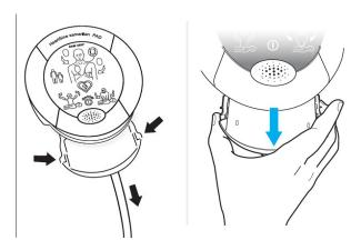
Once the Pad-Pak is removed from the device check the locator pins (blue arrows) to ensure they are straight and not bent, as shown in step 2 at the right.
